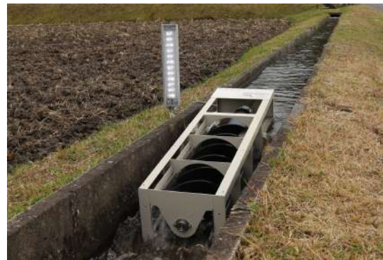
PicoPica 10 is structured with an appropriate elevation and a block plate to the inflow end and can be placed as it is on a flat and horizontal channel bed. The 6V LED light is a specially made auxiliary. It lights up when the generator is functioning normally. It can be used to light up the walkway or for security.
